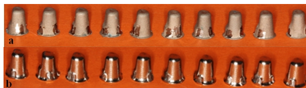
Figure 2a: CAD/Ceramill Sintron, b: CAD/Milling copings.
