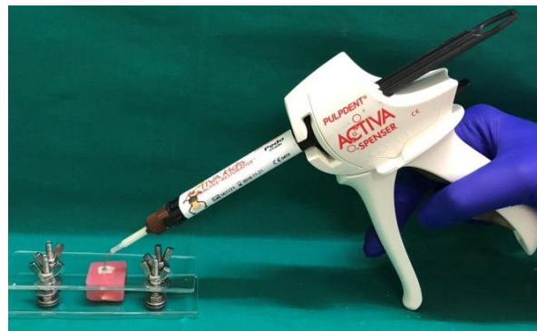
Figure 1: Dispensing ACTIVA KIDS using a spencer gun through the bonding jig template
