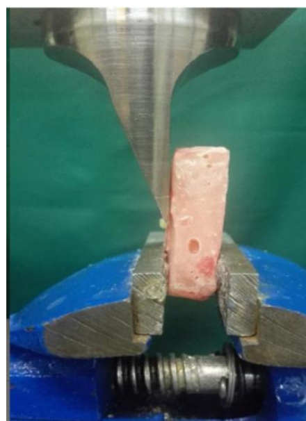
Figure 1: The specimen under the SBS test in the universal testing machine
