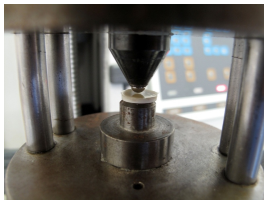
Figure 1: Arrangement for biaxial flexural strength test (Universal testing machine; LLOYD Instrument, Farham, UK).
