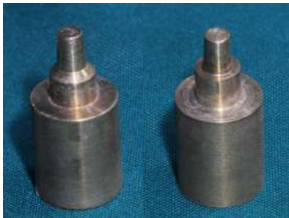
Figure 2a: Master die with 135° shoulder margin. b: Master die with 90° shoulder margin.
