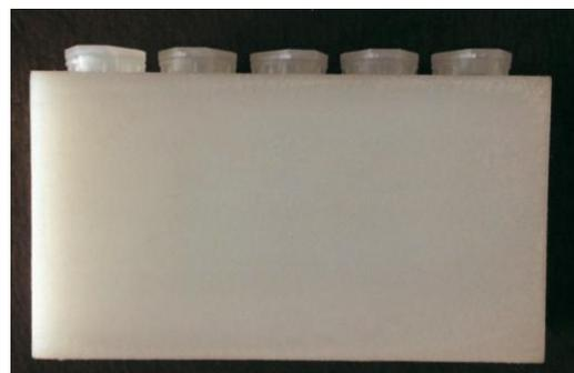
Figure 1: Polytetrafluoroethylene phantom
