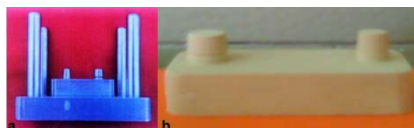
Figure 1a Stainless steel model with two dies: with undercut and without it on metal base b sample of stone cast
