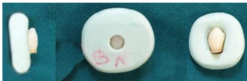
Figure 1: The putty mold used in this study for holding the test teeth to allow consistent measurement of L^* , a^* and b^* values
