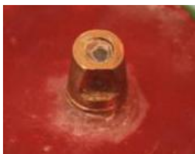
Figure 1: Brass die embedded in acrylic resin block
