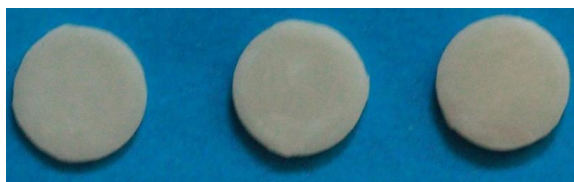
Figure 1: Monolithic zirconia disk specimens (from left to right: ceramic thicknesses of 0.6, 1.1, and 1.5 mm)
