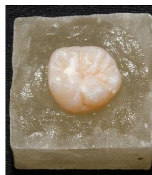
Figure 1: Molar tooth mounted in acrylic resin block
