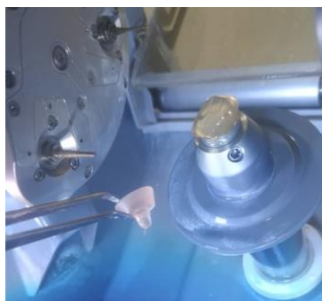
Figure 4: Semi-crystallized Suprinity endocrown before sintering
