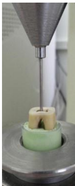
Figure 1: A specimen under push-out test using universal testing machine
