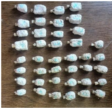
Figure 3: Teeth mounted in a mixture of type I stone and saw dust
