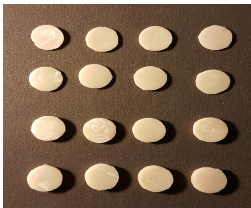
Figure 3: Group 2: Zirconia disks colored with A2 coloring liquid applied twice
