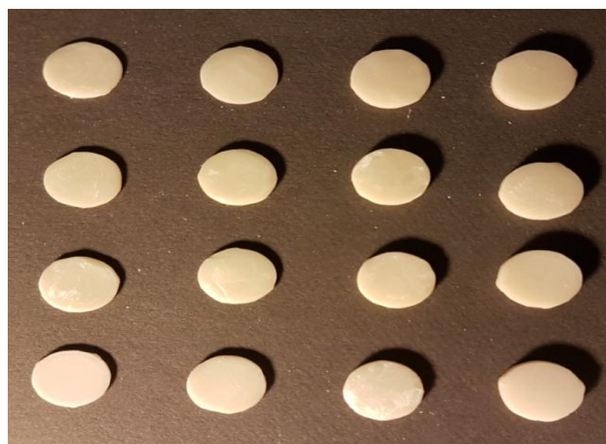
Figure 4: Group 3: Zirconia disks colored with A2 coloring liquid applied three times
