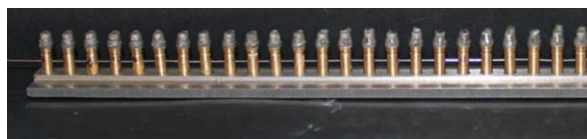
Figure 6 The specimens were aligned in a standard fashion after fixing on a machine-milled plate
