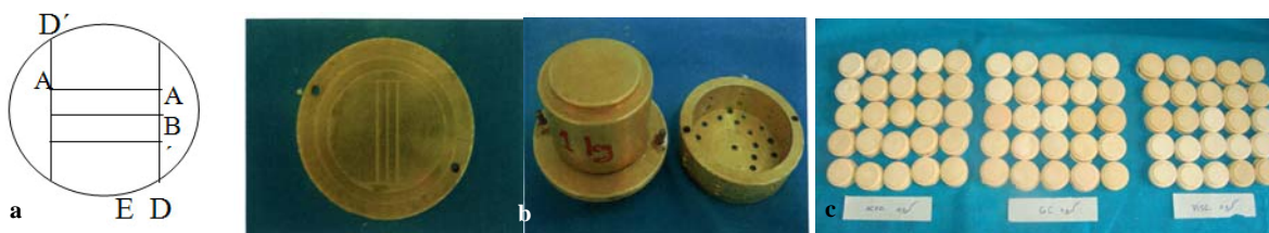
Figure 1a Schematic model b Ruled test block with 3 parallel liners and ring mold c Specimens of stones
