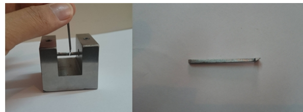
Figure 3: Metallic index to determine the gap angle
