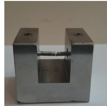
Figure 2: Custom device to hold the samples (lateral view)
