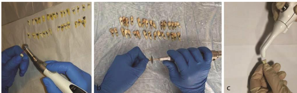
Figure 2: a: Cutting the crown of samples from 15 mm to Apex, b: Preparation of samples with rotary, c: Use of plasma device
