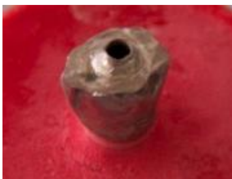
Figure 3: The ledge designed in the location of screw access channel of the third group of metal ceramic crowns
