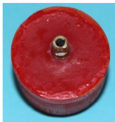
Figure 1: Brass die embedded in acrylic resin block
