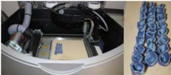
Figure 4: Wax-patterns fabricated by RP technology
